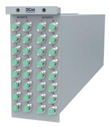
DiCon's **3D Matrix Switch Slot Card** is a proprietary optical switch that allows any of the inputs to connect to any of the outputs in a non-blocking optical cross-connect configuration. This innovative design is based on arrays of DiCon's industry proven MEMS mirrors, which redirect light from the input fibers to the requested output fibers. For ease of control, this 3D Matrix Switch is provided as a Slot Card for use in DiCon's GP850 modular system.
